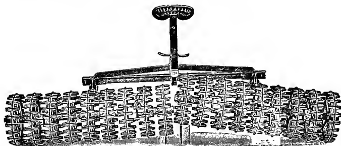
FIG. 71. "Clod crusher" and sub-surface packer.
